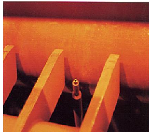
Between apron plate leaves in a hot plate mill
