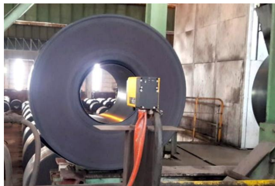
Detection of hot and cold coils
