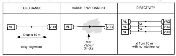
The emitter **VL** unit emits a high intensity, visible beam of modulated red laser light. This beam is received by a photosensitive diode fitted with an optical filter and whose signal is processed by the incorporated circuitry of the receiver **VRG**. The output changes state depending on whether the modulated beam is interrupted or not. Beam modulation, special optical filter and automatic correction make the sensor insensitive for ambient light.
